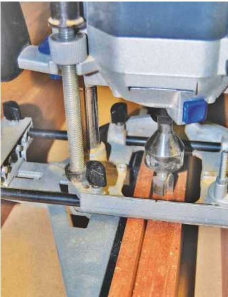
▲ Pic 4 ...but there's no reason why you can't do this on a router table. A router was used to cut the rebates
